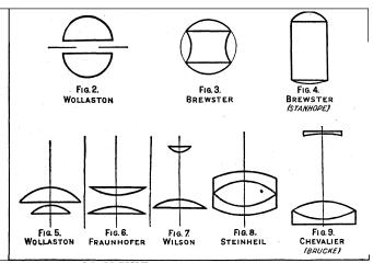
Figs. 2-9.—VARIOUS FORMS OF SIMPLE MICROSCOPES
