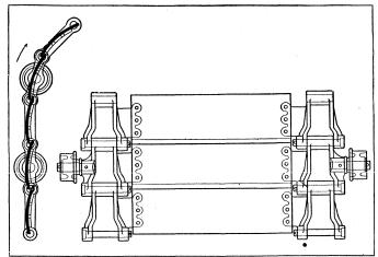
FIG. 6. — PORTIONOF APRON CONVEYOR WITH STEEL SLATS
