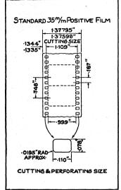
FIG. 1.-DIAGRAM SHOWING DIMEN. SIONS OF STANDARD 35MM. FILM
