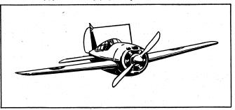
Fig. 2—THE Brewster all-metal fighter developed for the united states NAVY. The monoplane wing has no external bracing mestic civil use in the United States were monoplanes.
