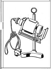
MICROSCOPE LAMP WITH BULL'S EYE AND SCREEN HOLDER
