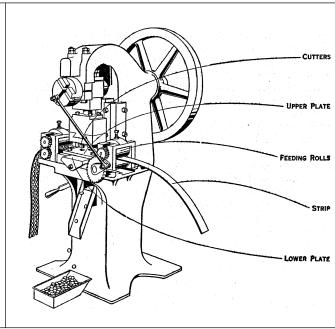
FIG. 1.— CUTTING MACHINE SHOWING HOW THE COIN BLANKS ARE BUNCHED, TWO AT A TIME, FROM THE STRIP OF SILVER BY THE DESCENT CYLINDERS
