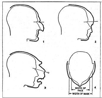
FIGS. 1-4 - DIAGRAM SHOWING SOME OF THE POSSIBLE VARIATIONS OF SIZE IN THE FACES OF MASKS
