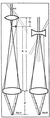
FIGS. 11 & 12. — DIAGRAMMATICREP-RESENTATION COMPOUND MI-CROSCOPES
