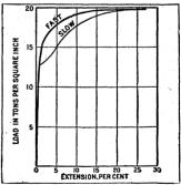
served to extend at first rapidly and then more slowly. In general it appears that the slow extension comes ultimately to an end; but when the applied load is nearly equal to that which would immediately break the specimen, the extension, after slowing down, quickens again and continues until rupture occurs. If, on the other hand, the specimen is subjected to an extension which is maintained constant, it is found that the load required to maintain that extension gradually diminishes.
