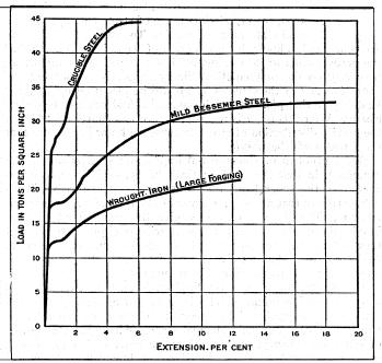
FIG. 11. — STRESS-STRAIN DIAGRAMS
