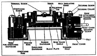
FIG. 3. — WESTERN ELECTRIC CONDENSER MICROPHONE
