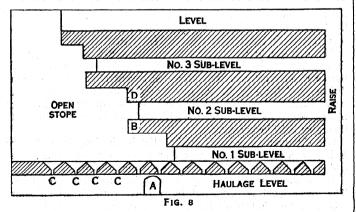
from slips. The sub-levels are carried back in steps, one working face being some 30 ft. horizontally ahead of that above.
