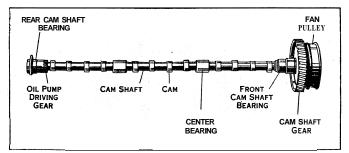
BY COURTESY OF GENERAL MOTORS CORPORATION FIG. 9. - CAMSHAFT
