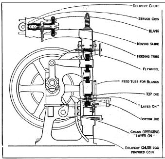
FIG. 2.—COINING PRESS SHOWING THE MASSIVE STRUCTURE OF A MODERN PRESS. WHICH RETAINS ITS RIGIDITY WHILE STRIKING A HEAVY BLOW EQUIVALENT TO A PRESSURE OF MANY TONS
