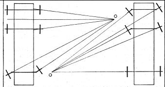
FIG. 2.—STEERING DIAGRAMS FOR SIX-WHEELERS
