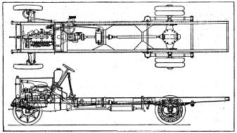
Fig. 1.—Thornycroft "Q' type chassis for loads of 5 to 6 tons
