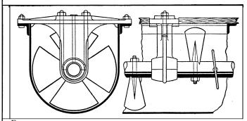
Fig. 2. — Portion of a paddle worm, showing steel trough and
