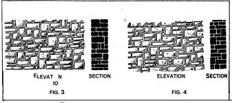
FIG. 3.— RANDOM RUBBLE WALLING FIG. 4. — COURSED RUBBLE WALLING
