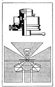
FIG. 23.— IMMERSION DAR K-GROUND ILLUMINATOR (BECK)
