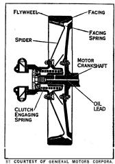
FIG. 14.—CONE CLUTCH
