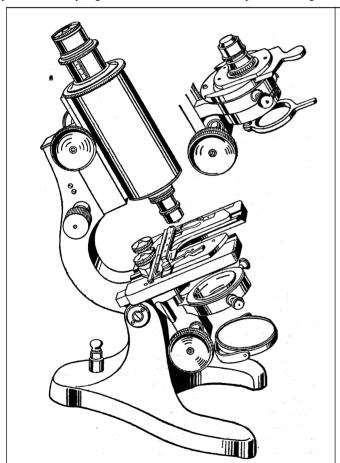
FIG. 22.— MICROSCOPE FOR GENERAL USE (BECK), SHOWING SUBSTAGE ARRANGEMENTS SEPARATELY IN THE SMALLER FIGURE
