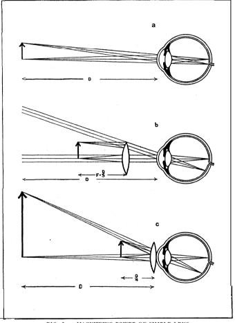
FIG. I. - MAGNIFYING POWER OF SIMPLE LENS (a) Object at distance of clearest vision (D), seen with unaided eye. (b) (a) Object at principal focus of a lens having focal length D/3. Image is at infinity. Magnifying power = 3. (c) Object so near to lens that the image is formed at distance D. Magnifying power, if the lens is in contact with the eye, =4
