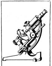
FIG. 2. — METALLURGICAL MICRO. SCOPE (ROSENHAIN TYPE), WITH FIXED BODY TUBE. HAVING THE ILLUMINATOR INSERTED IN 1T, AND MOVABLE STAGE
