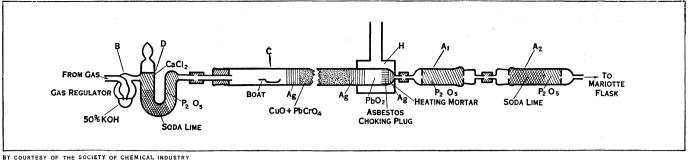
(B) BUBBLE COUNTER. (D) DRYING TABLE. (C) COMBUSTION TUBE. (H) HEATING MORTAR. (A,) WATER-ABSORBING TUBE. (A2) CAR-BON DIOXIDE-ABSORBING TUBE
