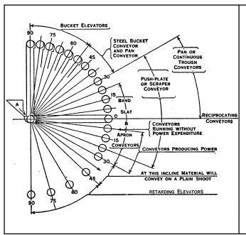
FIG. 9.— DIAGRAM SHOWING THE INCLINES AT WHICH VARIOUS TYPES OF CONTINUOUS CONVEYORS ARE APPLICABLE
