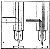
FIG. I. - DIAGRAM OF VERTICAL ILLUMINATION. A, TRANSPARENT REFLECTOR; B, OPAQUE REFLEC-
