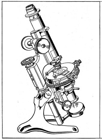
FIG. 25. — PETROLOGICALMICROSCOPE (SWIFT), AN INSTRUMENT FITTED WITH THE OPTICAL EQUIPMENT REQUIRED TO COVER A WIDE RANGE OF PETROLOGICAL WORK
