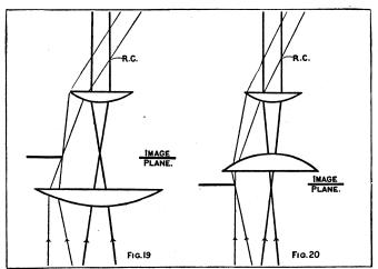
FIGS. 19 & 20.—PATHS OF RAYS THROUGH HUYGENS' EYEPIECE (FIG. 19). AND THROUGH RAMSDEN'S EYEPIECE (FIG. 20). R.C. DENOTING THE RAMSDEN CIRCLE IN EACH FIGURE
