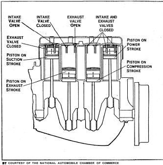
FIG. 2.— FOUR-CYCLE ENGINE CUT AWAY
