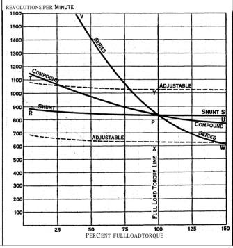
BY COURTESY OF THE WESTINGHOUSE ELECTRIC COMPANY Fig. 1.—CURVES showing the variation of speed with load of VARIOUS TYPES OF DIRECT CURRENT MOTORS
