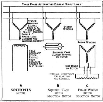
by courtesy of the westinghouse electric company  $Fig.\ 6$  — Schematic connection diagram for alternating current motors of the synchronous and induction types
